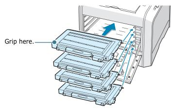
When the toner cartridges are correctly installed the yellow and black cartridges are not fully inserted. These will be pushed into place when you close the left cover.
